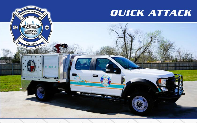
Chevrolet, Ford, or RAM Commercial Chassis 108" x 96" Custom Aluminum Body 5" Aluminum Mainframe, 4" Cross Members 3" x 3" Aluminum Headache Bar Full-Width 10" Rear Tailboard Step Custom Side-Body Compartments Swing or Roll-up Compartment Doors Custom Underbody Storage Compartments Hosebed Storage Compartment with Netting Rear-Body Access Steps Custom Painted Steel Bumper with Receiver PAC Equipment Mounting Options
